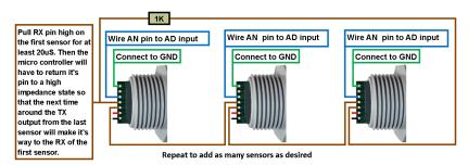
so on for all the sensor in the array. Once the last sensor has ranged, it will trigger the first sensor in the array to range again and will continue this loop indefinitely. Below is a diagram on how to set this up.
