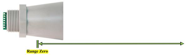
The range is measured from the front of the transducer to the target.
